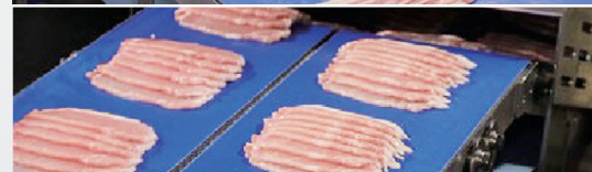
Dual type has individual conveyor control, which allows for fixed weight slicing of materials of different types and shapes at once
