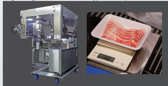
Dual type has individual conveyor control, which allows for fixed weight slicing of materials of different types and shapes at once
